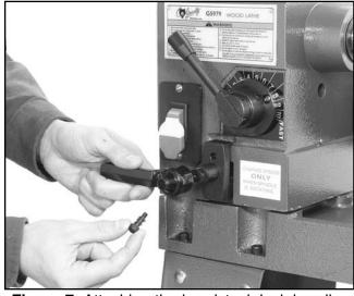
Figure 7. Attaching the headstock lock handle.
